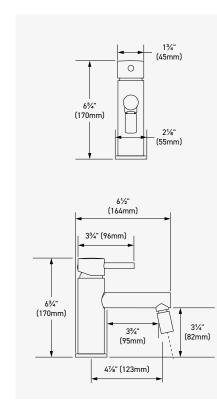
G 1/2" connection flexes. Supplied with G3/8" adaptor. Ceramic cartridge. Waste kit sold separately (DB160-EM). 8.3 I/min, 4 bar.
