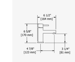
G 1/2" connection flexes. Supplied with G 3/8" adaptor. Ceramic cartridge. Waste kit sold separately (DB160-EM). 4.9I/min, 3 bar.
