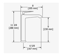
G 1/2" connection flexes. Supplied with G 3/8" adaptor. Ceramic cartridge. Waste kit sold separately (DB160-EM). 6.4I/min, 3 bar.
