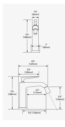
G 1/2" connection flexes. Supplied with G 3/8" adaptor. Ceramic cartridge.
