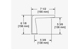
G 1/2" connection flexes. Supplied with G 3/8" adaptor. Quarter-turn ceramic cartridges. Waste kit sold separately (DB160-EM). 5.0/min, 3 bar.
