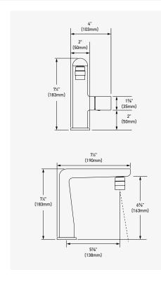
G 1/2" connection flexes. Supplied with G 3/8" adaptor. Ceramic cartridge. Waste kit sold separately (DB160-EM). 8.3 I/min, 4 bar.
