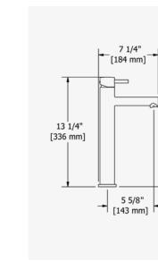
G 1/2" connection flexes. Supplied with G 3/8" adaptor. Ceramic cartridge. Waste kit sold separately (DB160-EM). 4.7I/min, 3 bar.
