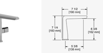
G 1/2" connection flexes. Supplied with G 3/8" adaptor. Ceramic cartridge. Waste kit sold separately (DB160-EM). 4.9/min, 3 bar.
