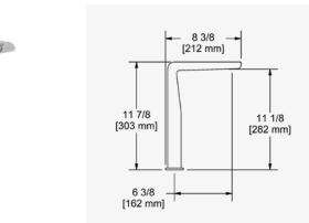
G 1/2" connection flexes. Supplied with G 3/8" adaptor. Ceramic cartridge. Waste kit sold separately (DB160-EM). 4.8/min, 3 bar.
