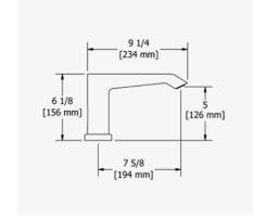
G 1/2" connection. Ceramic cartridge and balancing spool
